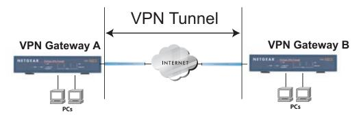
Figure 5-2: Gateway-to-gateway VPN tunnel
